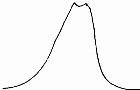
FIG. 8. Waveform of keying pulse at burst amplifier.
