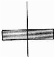
FIG. 6. Waveform of burst signal at input of phase detectors.
