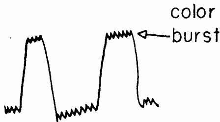
FIG. 7. Waveform of signal at grid of burst amplifier.
